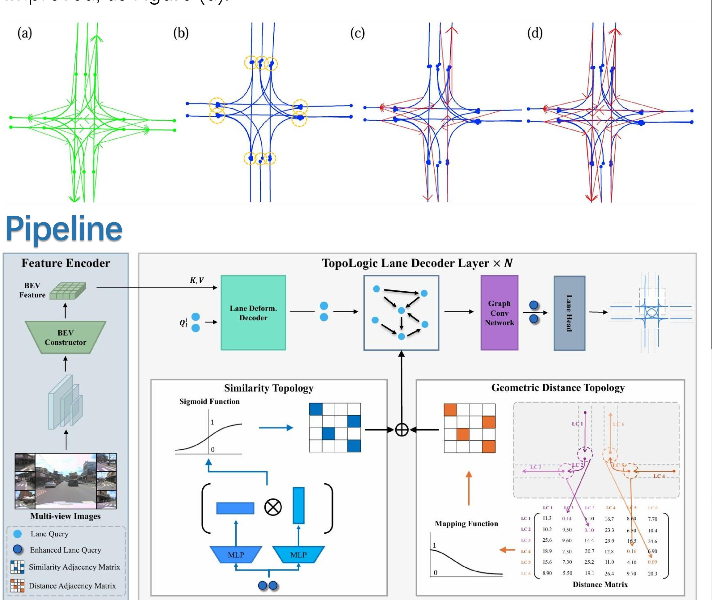
3. Lane Geometric Distance Topology: Consist of lane geometric distance matrix and distance to topology mapping function.
